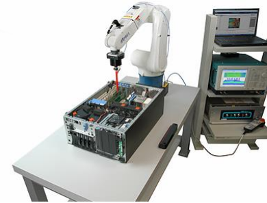
- Nearfield scanning test for debugging and analysis
