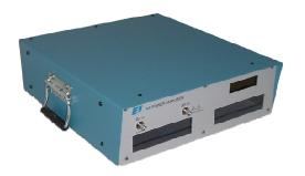
The 1020L Amplifier is a rugged source of RF power for ultrasonics, induction heating and laser modulation as well as plasma applications. It is a totally solid state solution employing RF DMoS FETs in the power amplification stages, offering simultaneous forward and reverse power readouts, and RS232 port for data collection. The 1020L reflects E&l's commitment to reliable and robust RF power.
