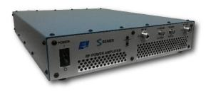
The 500S06 Amplifier is a rugged source of RF power for ultrasonic applications. It is a totally solid state solution employing Power MOSFETS in a full bridge PWM power stage. Operating at a significantly higher frequency than the fundamental signal
