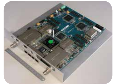
Q-Lite single card satellite modem
